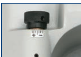
2 Tracer point with micrometric adjustment.
